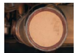
Above: Honeycomb particle trap from DPF on box truck. Left: Installation of a DPF simply requires replacement of muffler and tailpipe.
