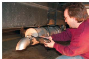
The combination of Diesel Particulate Filters (DPFs) and Ultra-Low Sulfur Diesel (ULSD) can achieve a 90% reduction in diesel particles.
